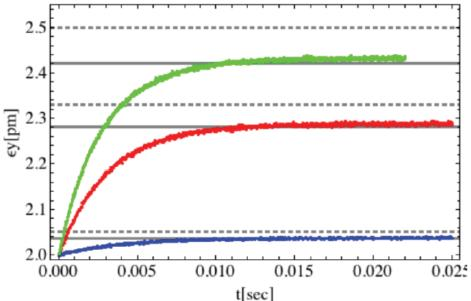
Evolution of horizontal, vertical and longitudinal emittances under the influence of IBS as obtained by the tracking code for different values of the bunch population: 6x10<sup>9</sup> (blue), 60x10<sup>9</sup> (red) and 100x10<sup>9</sup> (green). Horizontal lines represent the steady state values predicted by Piwinski (full) and Bane (dashed) models for the considered bunch populations.
