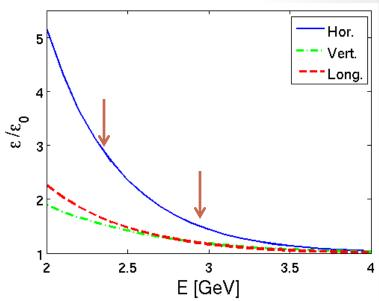
Broad minimum of the emittances around 2.5 GeV (left) while the IBS effect becomes weaker with energy (right)
