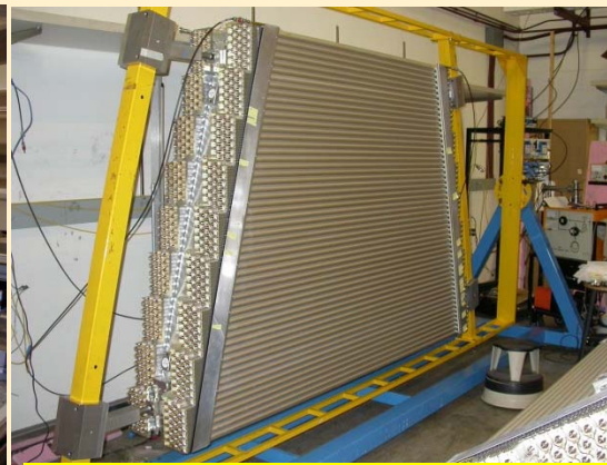
Completed endcap chamber
