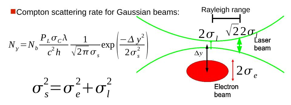
By measuring Compton rate (N<sub>y</sub>) as a function of relative displacement (Δy), the quadrature sum of the beam sizes (σ<sub>s</sub>) can be determined
