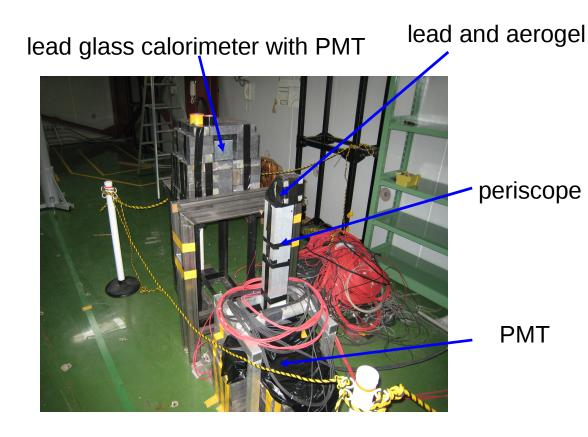
2 detectors for measuring the LW Compton rate (N)
