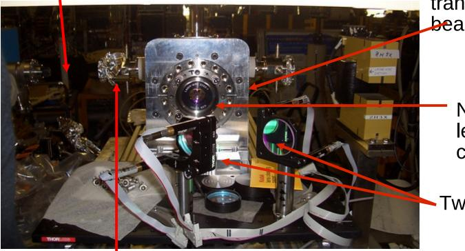
Chamber can now be moved along 2 axes transverse to electron beam
