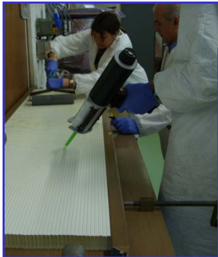
Applying glue to sides of bars
