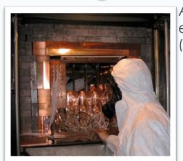
As a result of a 2nd generation R&D for more radiopure NaI(TI) by exploiting new chemical/physical radiopurification techniques (all operations involving - including photos - in HP Nitrogen atmosphere)
