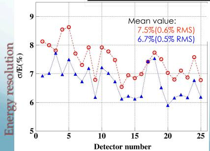
$\sigma/E$  @ 59.5 keV for each detector with new PMTs with higher quantum efficiency (blu points) and with previous PMT EMI-Electron Tube (red points).
