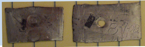
Lead shims with ^{210}\text{Pb}
