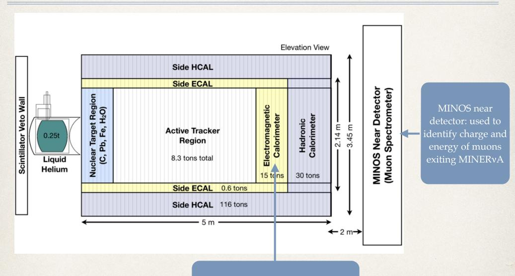
EM Calorimeter is scintillator + lead. Used as part of calorimetric recoil measurements.
