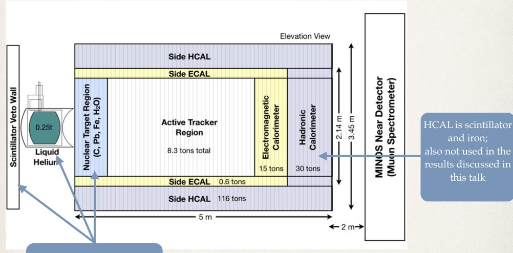
Passive targets and veto wall will be used to compare cross sections across different nuclei in the future, but are not used in today's work.
