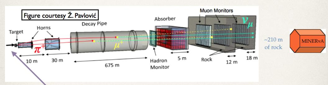
The NuMI neutrino beam starts with a 120 GeV proton beam from Fermilab's main injector
