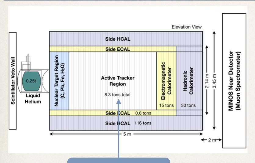
The MINERvA detector is made of 120 "modules" of varying composition.
