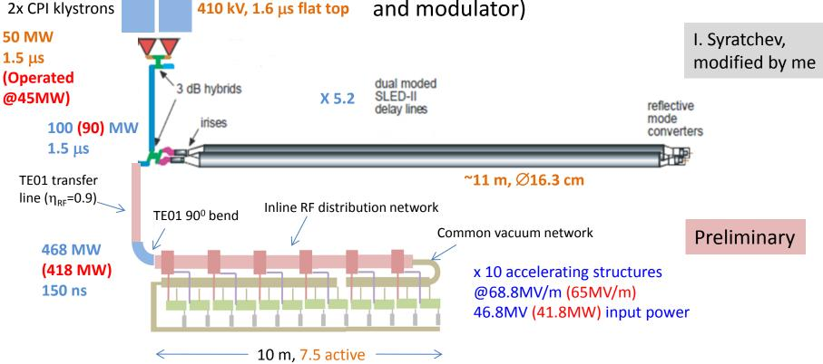
This unit should provide ~516 (488) MeV acceleration beam loading. Need 12 (12) RF units. Cost 51.7 a.u., 4% more than optimum
