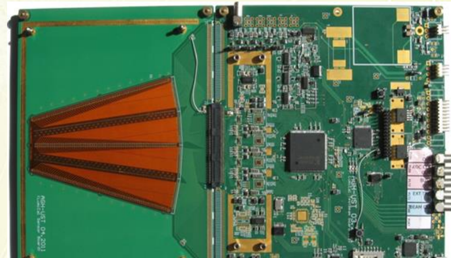
Fully assembled sensor plane, ready for testbeam studies
