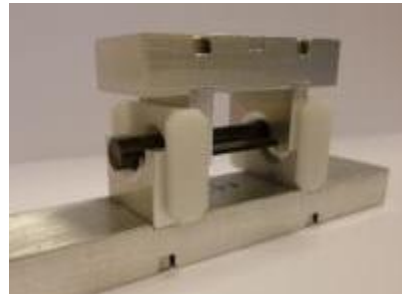
4 points bending test on rods
