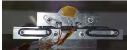
4 points bending test on plates
