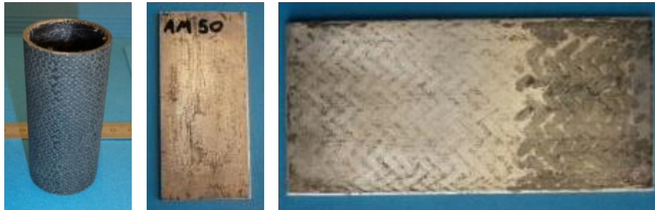
Tube and plates of long carbon fibres in aluminium matrix
