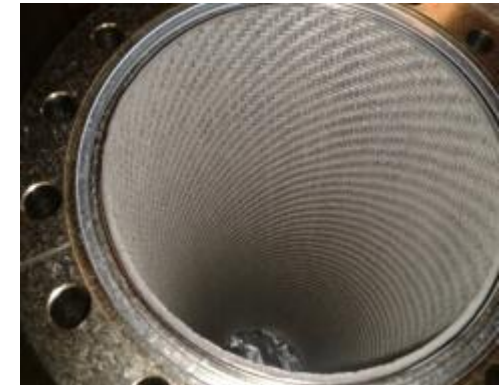
Internal C/C tube
