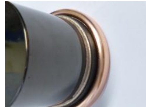
GC crucible soldered with a copper ring
