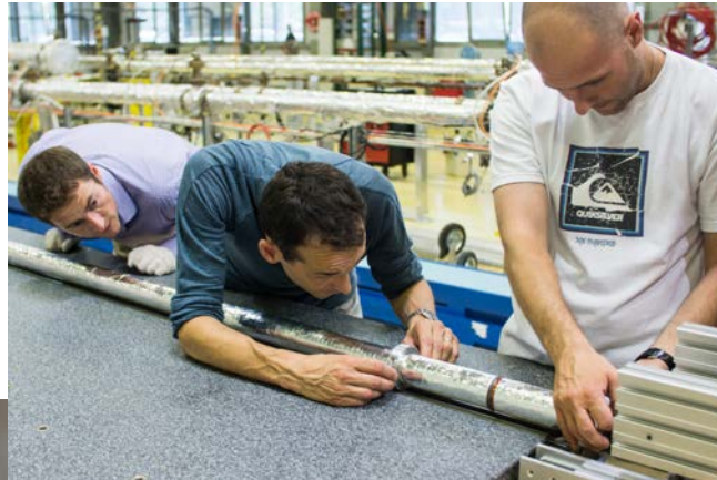
Transfer of beampipe to support
