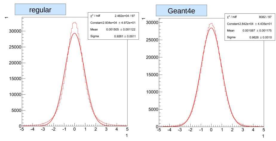
The Geant4e material model is able to achieve a slightly better mean (0.0015 vs. -0.0010) and sigma (0.926 vs. 0.983) than the regular method
