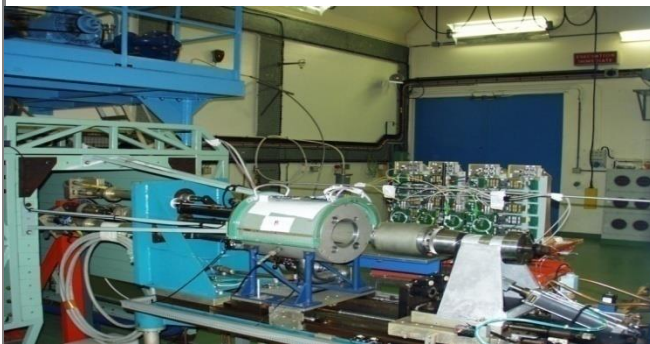
1 MeV neutron displacement damage tests
