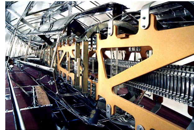
Vivitron, Straßbourg, inner structure of the acc. section
