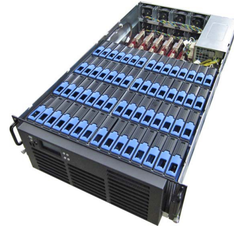
Foxconn's 4U Storage Server with 60 drives
