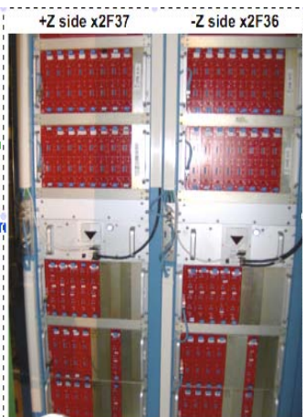
CAEN A4603 power supplies (PS) Modified to be compatible with DC-DC conversion
