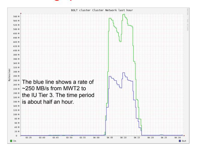
The green line is twice the data rate from MWT2 because the plot shows the aggregate rate data rate for the IU Tier 3 and internal transfers and external transfers are combined on the plot.
