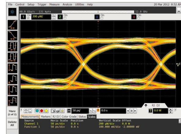
Eye diagram @ 4Gbps. 53 cm line including SMA cables.
