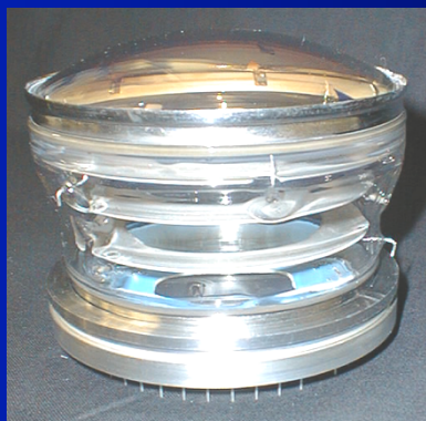
HPD tube manufactured at CERN: 2048 channels
