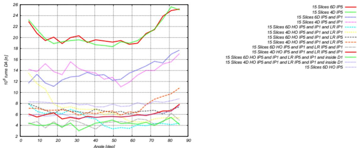
Differences 4D vs 6D (always referred to BB lenses) coming from adding second LR set. Optics used round 10/10 cm. Possible hints large amplitude more affected in 6D (growing tails), synchrotron resonances effect, simply numerical issues due to different implementation.
