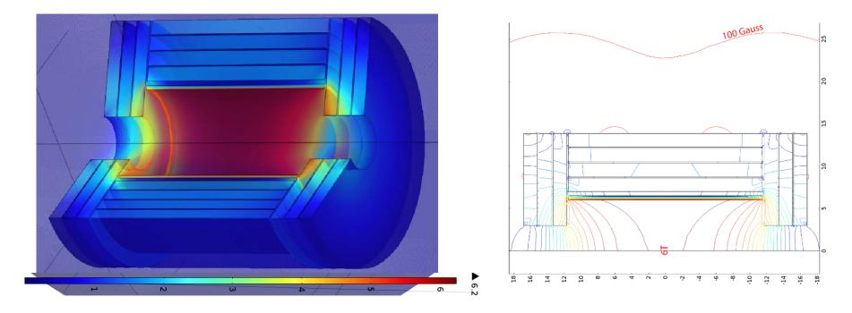
6 T in a 12 m bore, 23 m long, 28 m outer diameter.
