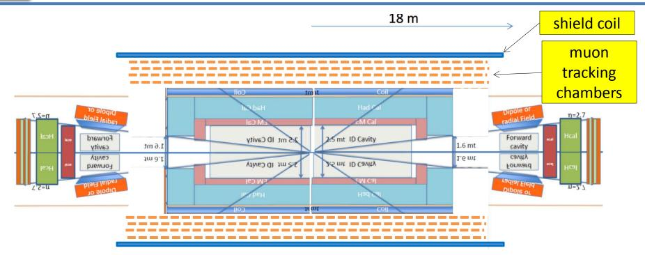
Twin Solenoid: the original 6 T, 12 m x 23 m solenoid + now with a shielding coil {concept proposed for the 4<sup>th</sup> detector @ILC, also an option for the LHeC in the case of large solenoid; and this technique is in all modern MRI magnets!}.
