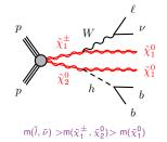
Searched for events with one charged lepton  $(e,\mu)$ , missing transverse momentum and 2 b-tagged jets consistent with a Standard Model Higgs boson at  $m_H = 125 \text{ GeV}$
