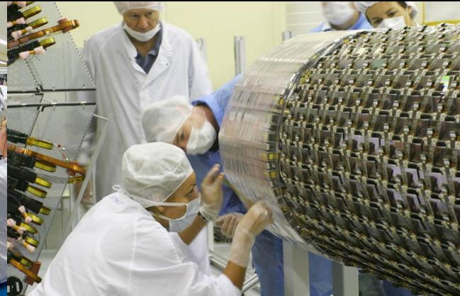
**Electromagnetic Calorimeter  $|\eta| < 3.2$**
