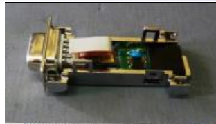
RADMON PCB BASED WITH 2 RadFETS DETECTORS 1xLAAS 1600 - till 10 Gy 1xREM 250 - till 2000 Gy
