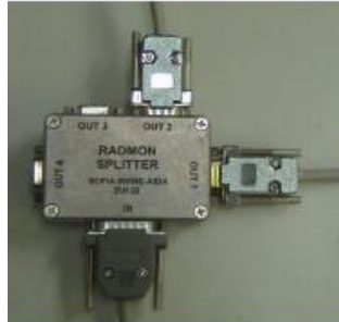
FOUR DETECTORS CAN BE CONNECTED TO ONE SPLITTER BY SHORT CABLES THE SPLITTER IS CONNECTED TO THE DETECTOR NODE BY A LONG CABLE
