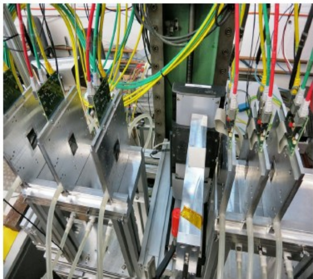
Top-bottom view on the EUDET telescope sensor fixtures with a DUT box mounted in between. (Photo by CLICpix group at DESY testbeam)
