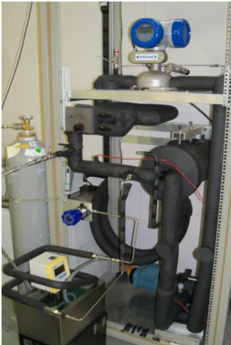
Pump test stand for endurance tests
