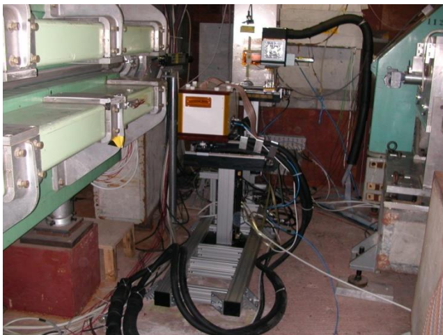
First production 3axis scanning table with cold box (above). Scanning table and rail system installed in beam line (below)
