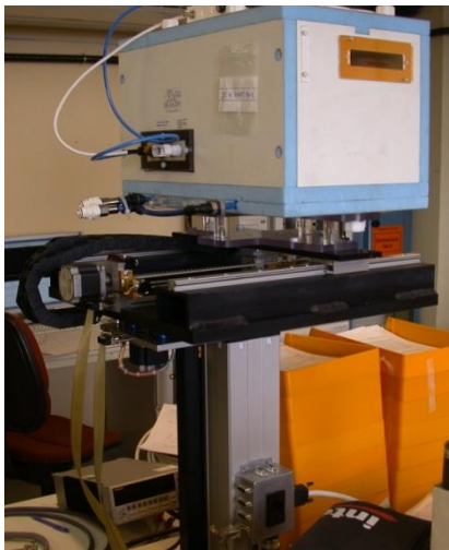
First production 3axis scanning table with cold box (above). Scanning table and rail system installed in beam line (below)
