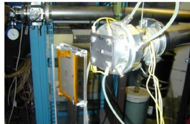
Alignment complete, Ni foils marked for position prior to 1 st run.
