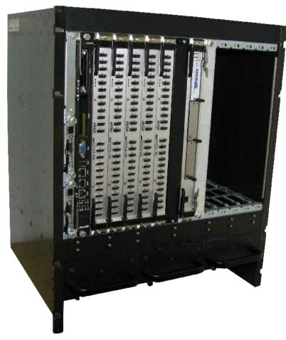
Only system at CERN has all boards running, all others ADC boards have to be re-work
