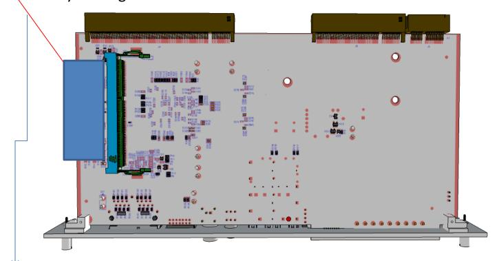
This required complete re-routing of critical DDR3 lines, pin swapping ect by UPV First PCBs and final component list ~ End Nov 2013...
