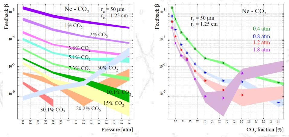
✤ Photon feedback parameters decrease with increasing pressure and admixture fraction till 20.2% CO<sub>2</sub> (related with the mean free path of the photons),
