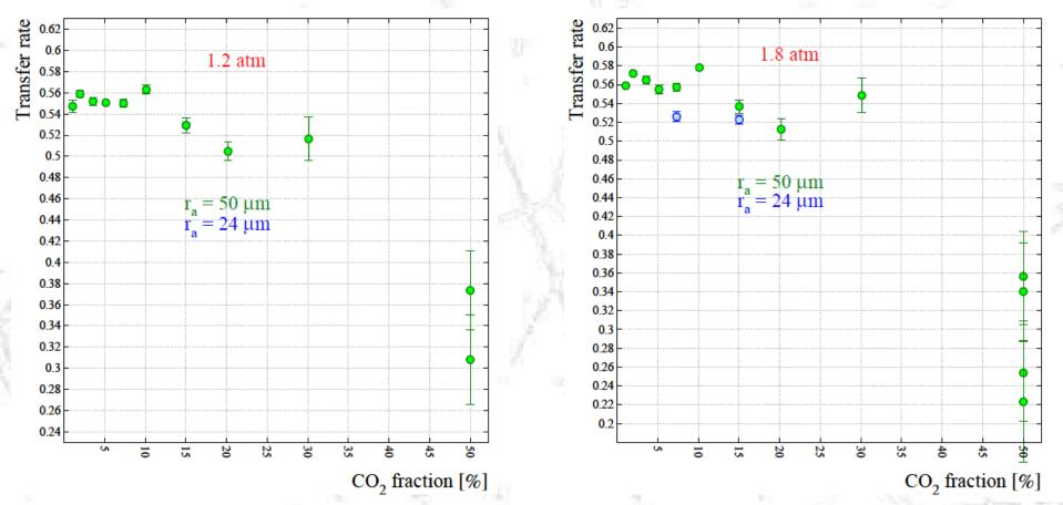
The biggest transfer rate shifts to 10% CO<sub>2</sub> (both at 1.2 atm and 1.8 atm),
