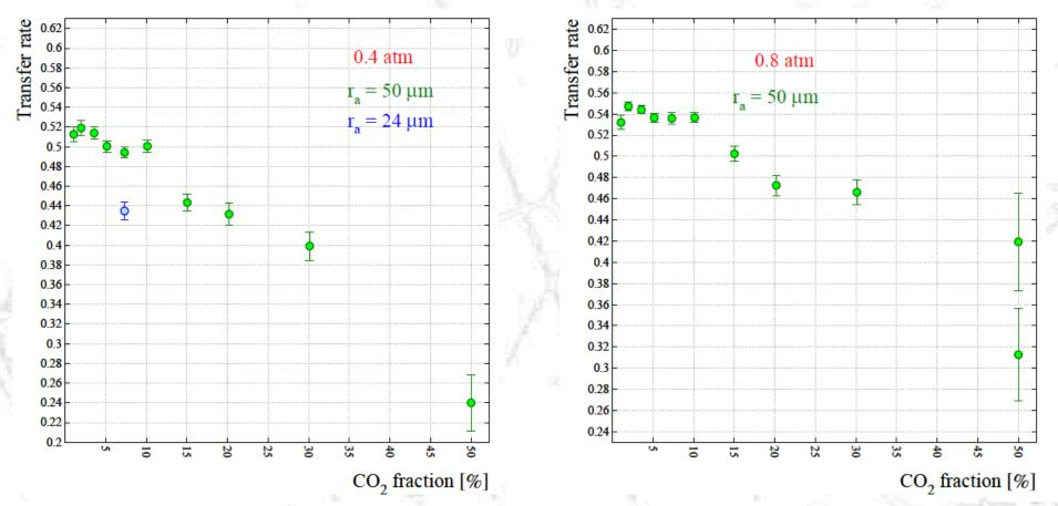
\* The biggest transfer rate for 2%  $CO_2$  (both at 0.4 atm and 0.8 atm),
