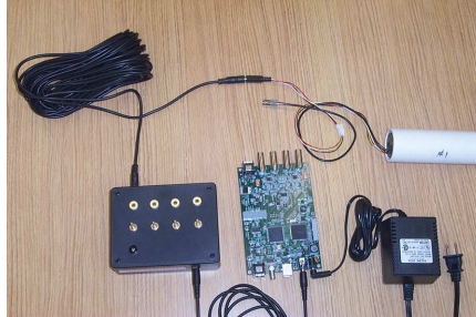
3. PMTs/counters (4) PDU (four, side outlets): 50 ft. power extension cable, stereo connectors
