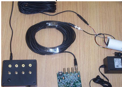
4. PMTs/counters BNC connections (4) DAQ BNC connections: 50 ft. BNC signal ext cables
