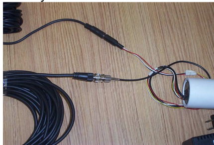
4. PMTs/counters BNC connections (4) DAQ BNC connections: 50 ft. BNC signal ext cables
