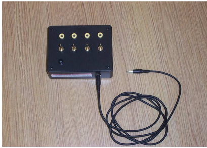
2. DAQ female jack PDU (single, side outlet): 6 ft. PDU power cable, male mono connectors
