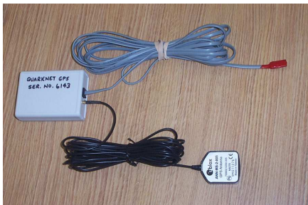
5a. GPS antenna GPS Receiver Assembly: black MCX cable 5b. temp sensor GPS Receiver Assembly: gray phone cable, red sensor end 5c. GPS Receiver Assembly DAQ: CAT-5 green network cable Note: CAT-5 cable plugs into DAQ "GPS IN", not "GPS FANOUT".
