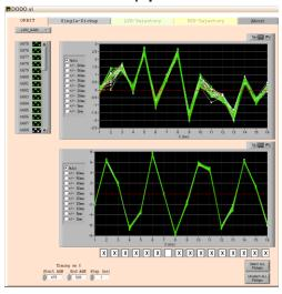
Orbit after correction (up to 1.6 mm in vertical)
