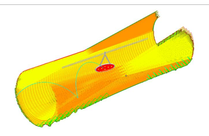
High granularity Less material High Trasparency DC towards the TC counter  $\sigma(E_e) \text{ [keV]} \sim 150 \text{ (325)}; \\ \sigma(\theta_e, \Phi_e) \text{ [mrad]} \sim 5 \text{ (7-11)}; \\ \epsilon(\text{det)} \text{ [\%]} \sim 80 \text{ (40)}; \\ \sigma(t_e) \text{ [ps]} \sim 30 \text{ (70)};$
