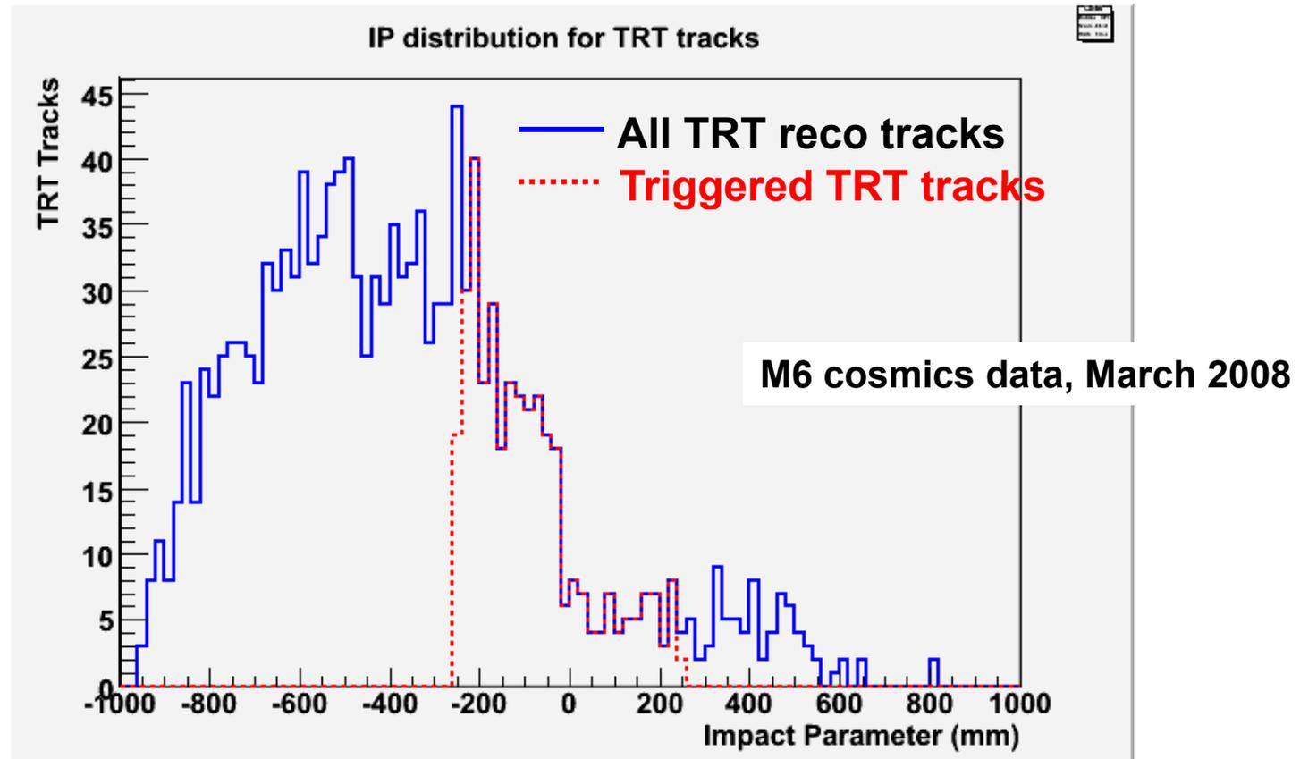
The trigger required TRT tracks reconstructed online within the pixel volume (equiv. to impact parameter  $\leq 25$  cm around zero)
