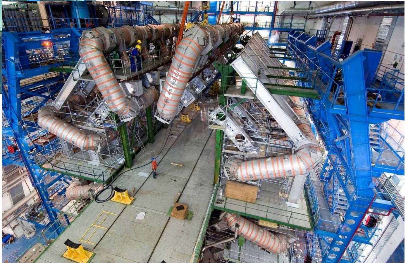
The last coil was moved into position on 25 th August 2005
