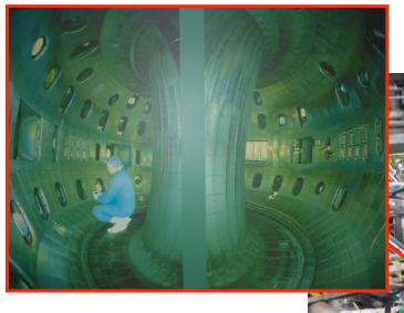
2.1 tesla torus (normal-conducting coils)
