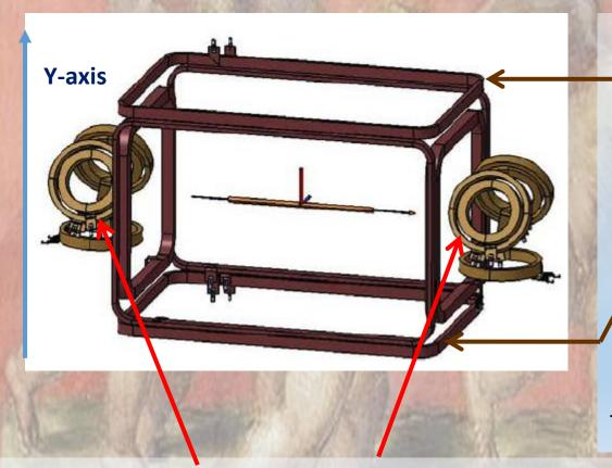
Spin filtering in transverse case, quantization axis, defined by the top and bottom, Holding field coils.
