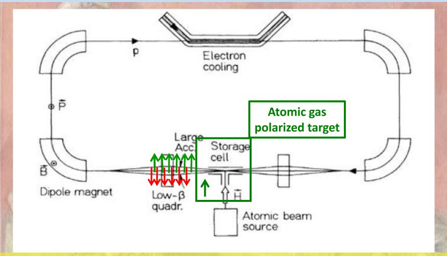
An un-polarized beam by multiple passage through a polarized target, due to different cross-section for parallel ( $\uparrow \uparrow$ ) and antiparallel ( $\downarrow \uparrow$ ) spin alignment, becomes polarized, while the intensity decreases.
