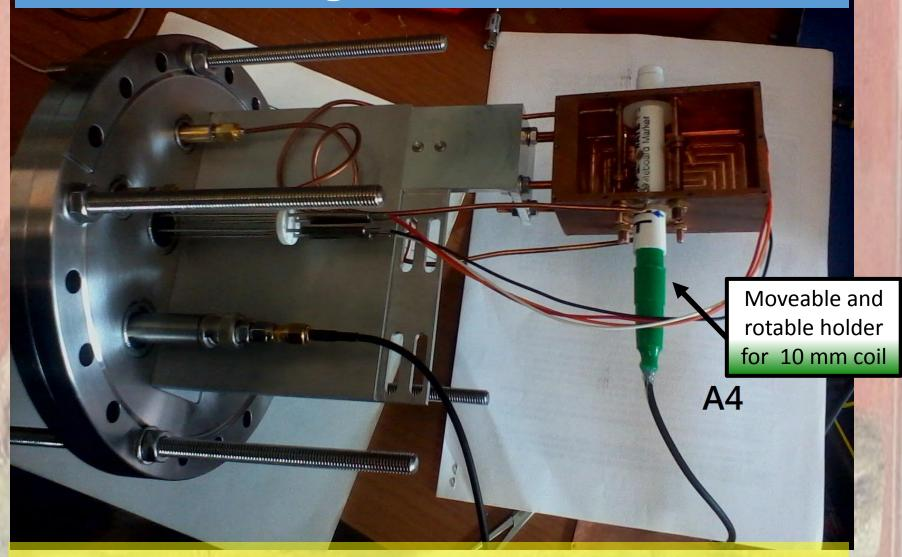
Check on  $45^{\circ}$   $B_{rf}$  and adiabatic transition conditions.
