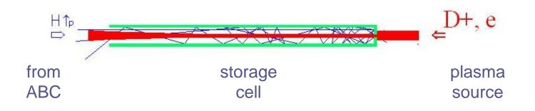
11 mA of H<sup>+</sup>↑ 80 % polarization has been obtained from the INR source
