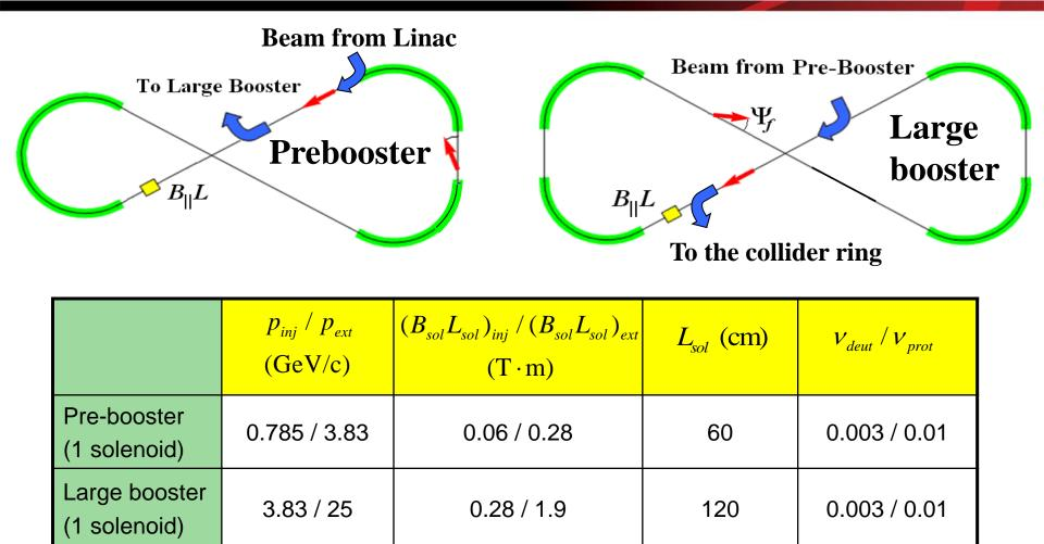
Conventional 20 GeV accelerators require  $B_{\parallel}L$  of ~70 Tm for protons and ~250 Tm for deuterons
