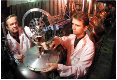
Internal Target Station is very well suited for the measurements of the deuteron- induced reactions observables at large scattering angles.
