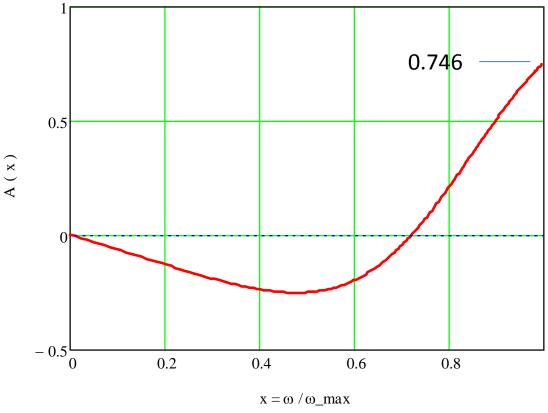
The longitudinal Compton polarimeter should be used due to its huge sensitivity to the longitudinal component of the polarization. Detection of the scattered electrons provides excellent spectral selectivity to their energy loss. Thus, one can use events near the spectrum edge!
