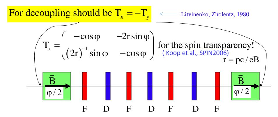
Two solenoids, each L=40 m B=5 T, provide spin rotation by  $\phi = 180^{\circ}$  at E=45.5 GeV. Extension to 120 GeV with B=10 T looks feasible.
