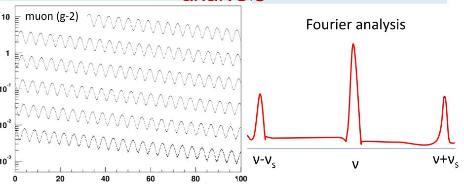
Could be observed also other peaks, for example, from coherent betatron oscillations. But the central line will dominate always.
