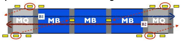
Re-location of 2<sup>nd</sup> position quadrupole BLM to the close-by dipole-dipole interconnection
