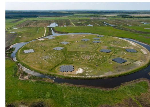
LOFAR superterp (Netherlands) – 21x96 antennas – \phi = 350 m
