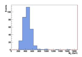
Z' generated @ 500 GeV. Reconstruction of M<sub>Z'</sub>
