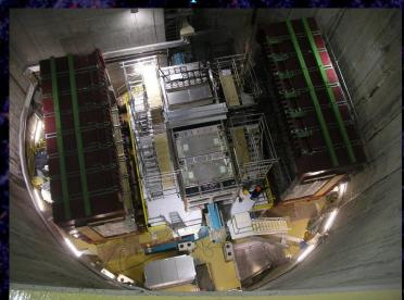
T2K 280m near detectors, will be re-used, but upgraded (?) and maybe enhanced with new near detector(s) at 2km.
