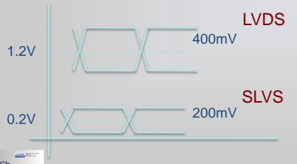
SLVS specifications brief 2 mA Differential max Line impedance: 100 Ohm Signal: +- 200 mV Common mode ref voltage: 0.2V
