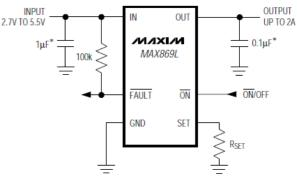
Hight speed current increase ⇒ Output is switched off during few ms
