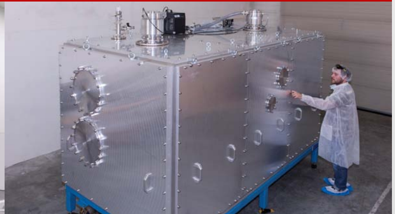
Compressor and vacuum chamber
