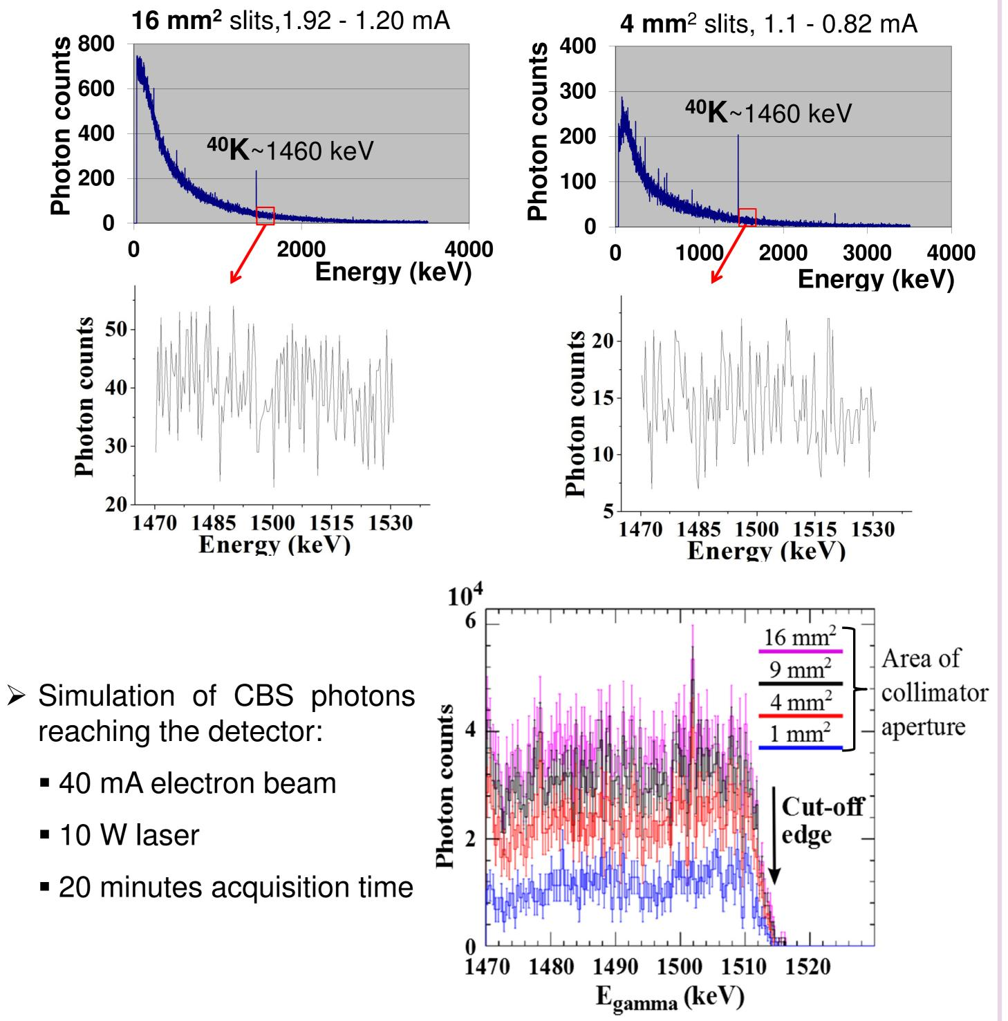
$\succ$  High purity Ge (HPGe) spectrometer: high energy resolution (~10<sup>-3</sup>).  $\succ$  CW CO<sub>2</sub> laser (wavelength 10.6 µm, E<sub>1</sub> 0.117 eV): E<sub>max</sub> is within the sensitivity range of commercially available HPGe spectrometers.
