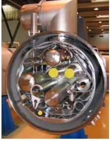
Finished SSS 233, with vacuum barrier: a long story of leaks and repairs (bulk material leak). Successful final pressure test!
