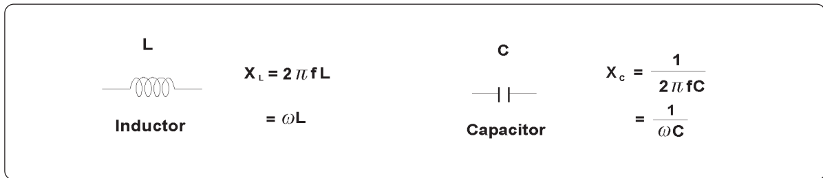
Figure 1-3. Reactance in two forms: inductive ( X_L ) and capacitive ( X_C )
